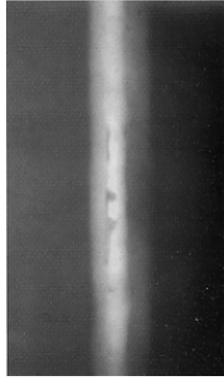
Lack of side wall fusion with slag
